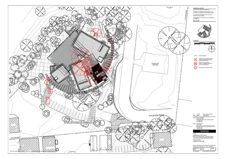
**Figure 3** - Schematic Ground Floor Site Plan of proposed buildings and associated infrastructure comprising the Resource Recovery Learning Centre at Flatrock Road, Mundamia with trees to be retained and those to be removed as well as landscaped tree plantings indicated at the site and surrounds (Terroir Architects 2023)
